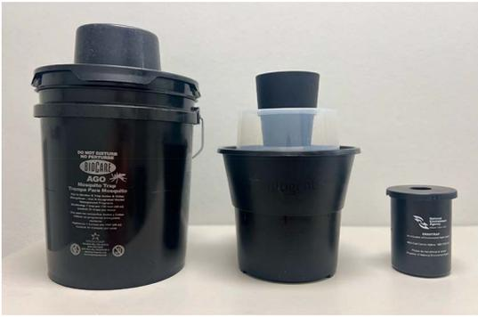
Fig. 1. Traps used for comparison study (left to right): CDC Autocidal Gravid Ovitrap (AGO), Biogents Gravid Aedes Trap (GAT), and Singapore Autocidal Gravid Trap (SGT).
