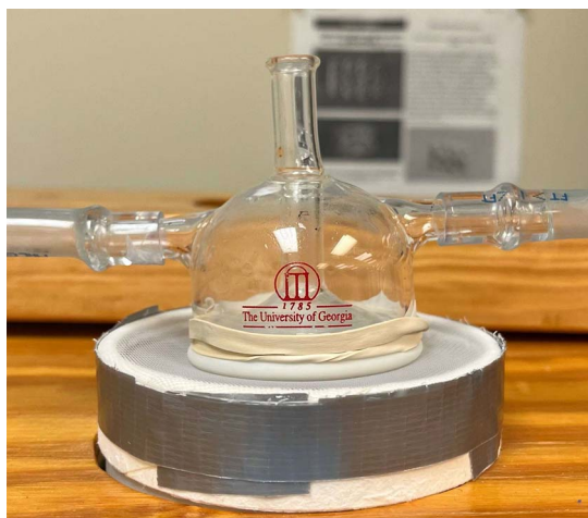
Fig. 1. One of 4 water-jacketed membrane feeders with fittings on either side and a top port for addition of liquid. The feeder is affixed with a latex membrane and set atop an adult feeding container. The nylon mesh top is pulled tightly to support the weight of the feeder, while enabling flies to feed through it.
