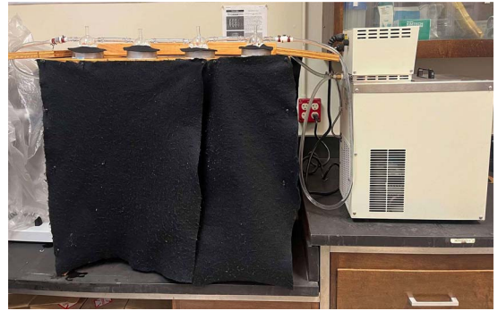
Fig. 3. The water-jacketed membrane feeder apparatus and viewing frame. The connected water-jacketed membrane feeders sit atop 4 adult feeding containers loaded with 40 female flies each and connected to the water bath on the right of the image. The viewing frame supports the apparatus and is shrouded below and on top.
